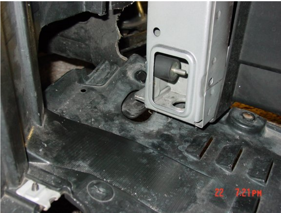
A test fit of the CAI main pipe. At this point I decided to remove two plastic button-type clips holding part of the second undertray.
