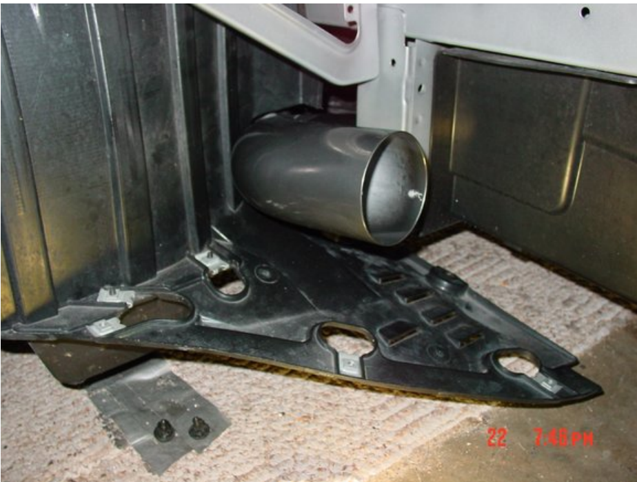
Here are two shots showing both undertrays partially loosened and hanging loose, with the CAI pipe in position.
