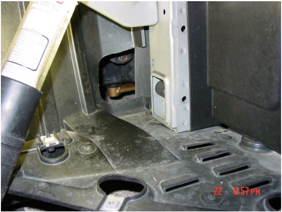
The next three pictures show how I used a hole saw to get a good start on cutting most of the other plastics.
